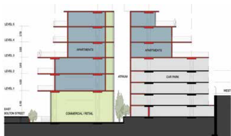
Figure 4.46 Bolton Street carpark - proposed section (TZG 2012)
